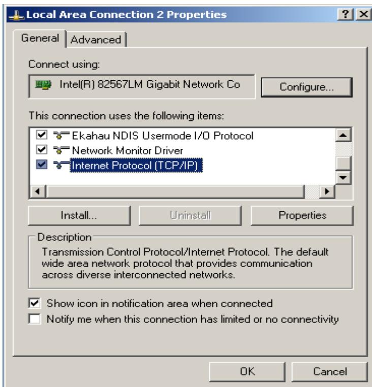
4. Pada paparan seterusnya, pilih “***Obtain an IP address automatically***” dan “***Obtain DNS server address automatically***”. Seterusnya klik ***OK***.
